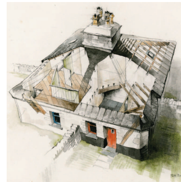
Falcon Hildred's superb record drawing from 1978 of four conjoined quarry workers' houses built in 1810 at Blaenau Ffestiniog, Tai Uncom. FHA 01_143_01, NPRN 28880.
